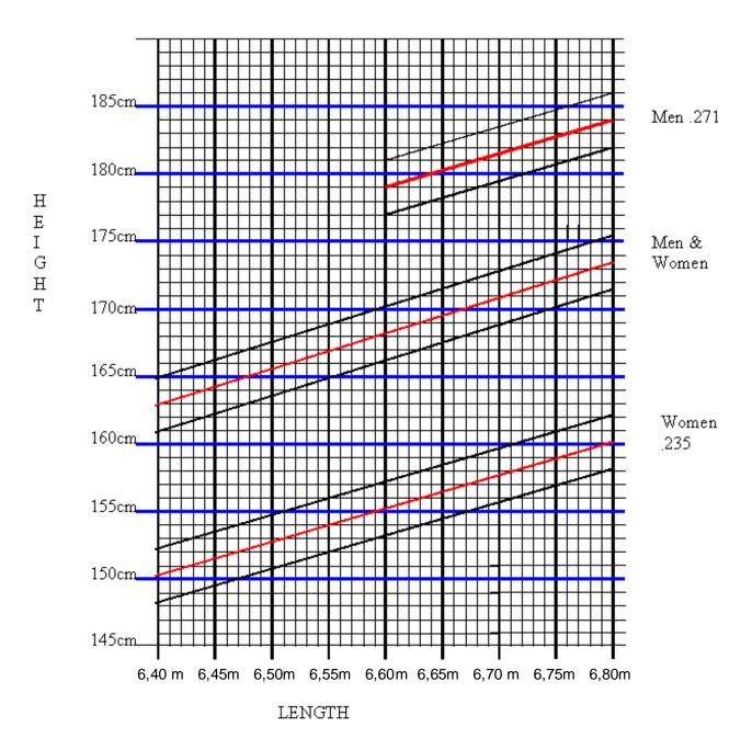
Instructions: For any particular ramp setting, a combination of HEIGHT at the top edge and LENGTH out of the water enclosed within the solid line is allowable. A combination that lies on the dotted (middle) line is the most desirable.
