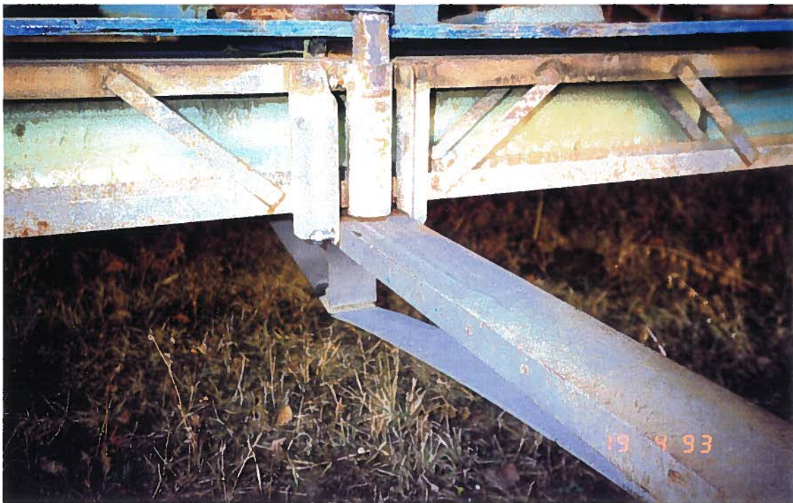
FRONT TRAILER TRUSS WITH TOWING BAR IN POSITION. ALSO BOAT BUMPER AND SLEEVE SHOWN IN POSITION.
