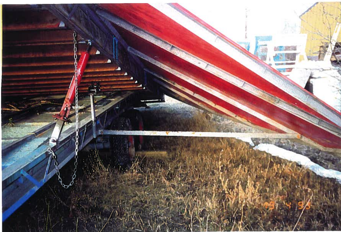
WIDE ANGLE OF LEFT SIDE OF TRAILER, DECK AND WING. NOTE SAFETY CHAIN. HYDRALIC JACK IS NOT MOUNTED IN ACCORDANCE WITH DESIGN RECOMMENDATIONS. NOTE WING BRACKET WELDED TO DECK FRAME.
