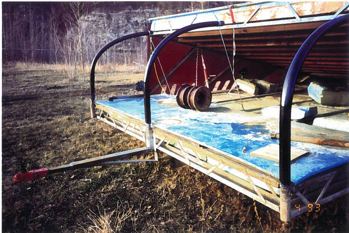
FRONT OF JUMP. NOTE WORKING DECK AREA 4' X 12'. ALSO UNIQUE DRIVETRAVING BOAT RIMMED SLEEVES
